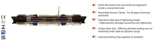
The **501/RCG Coupler** is certified Exe, and is an inline quick connection product suitable for use as a cable extension device or an alternative to a junction box. Suitable for all types of cable, including unarmoured, armoured and braided.
