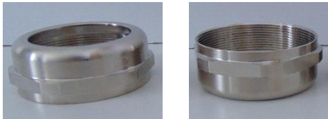
Figures 3 and 4: Sample 2a "Part 50.663 M, PERFECT cable gland made of brass CuZn39Pb3 as per EN 12164, surface nickel-plated", different perspectives.
