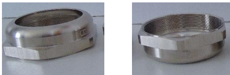
Figures 7 and 8: Sample 3a "Part K150-1063-00, WADI one cable gland made of brass CuZn39Pb3 as per EN 12164, surface nickel-plated", different perspectives.
