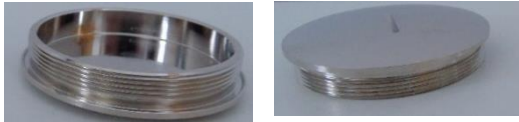
Figures 1 and 2: Sample 1 "Part 10.7515 M/G, Screw plug made of brass CuZn39Pb3 as per EN 12164, surface nickel-plated", different perspectives.
